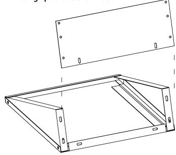
**5.** Fasten the back to the sides with four #8-32 x <sup>1</sup>/2" bolts (Ref. No. 5) and nuts (Ref. No. 6).
