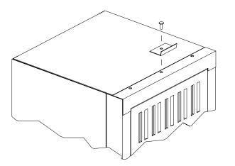
NOTE: On some locker units, the existing hole may contain a rivet. If so, use a drill with a <sup>3</sup>/16" bit to remove the rivet before installing the clips.
