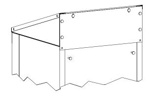
**12.** Tighten all hardware. Don't forget to tighten the nut under each retaining clip. Your sloping top is now installed.
