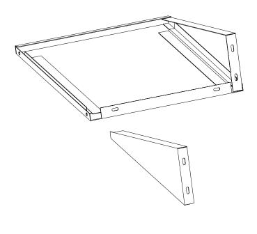
**4.** Place the back plate (Ref. No. 3) against the flanges on the outside of the top and sides.
