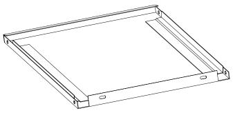
**3.** Slide the right and left side plates (Ref. No. 2) into the front retaining strips of the top plate.
