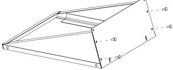
6. Fasten the back to the top along the return bend using two #8-32 x 1/2" bolts and nuts on a single wide unit, or four #8-32 x 1/2" bolts and nuts on a three wide unit.
