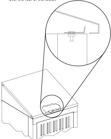
**10.** Using a drill and <sup>3</sup>/16" bit, drill two holes through the holes in the back plate and into the rear of the locker.
